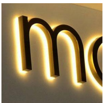
4. ACRYLIC INDIVIDUAL LETTERS WITH METAL COATING PINNED OFF WALL WITH HALO LED (CONCEALED) LIGHTING BEHIND, SHOP SIGNAGE
