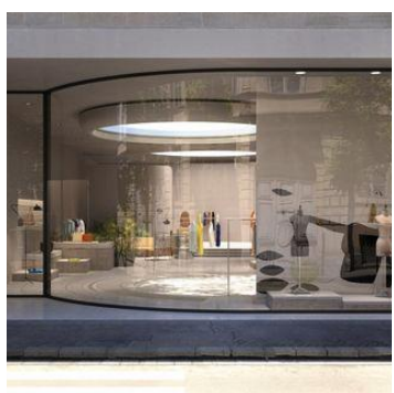
6. ANODISED ALUMINIUM WINDOW/DOOR FRAMES TO MATCH 3, SHOP FRONT WINDOWS (CLEAR SAFETY GLASS)
